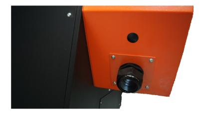
Pass the cable into the electrical cabinet and connect the 3 phases, the neutral and the earth
