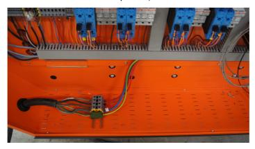
Unlock all the emergency stop buttons If this LED is lighted ON, switch the phase 1 and 2 If it stay ON, one phase is missing
